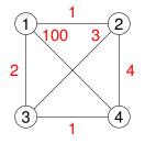
$$C = (c_{i,j}) = \left[ egin{array}{cccc} 0 & 1 & 2 & 100 \ 1 & 0 & 3 & 4 \ 2 & 3 & 0 & 1 \ 100 & 4 & 1 & 0 \end{array}
